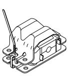
Make sure the tie-wraps are holding firm while releasing the clamp or vise. The metal shells may separate slightly, this is normal. However, excessive separation will cause the mounting bolts to not reach through the crossmember and allow the nuts to start on the bolts. Cut the ends of the tie-wraps off, being sure not to leave any sharp edges.
